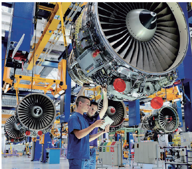
图2 CFM56发动机的脉动装配生产线 Fig.2 Pulsating production line for CFM56 engine
