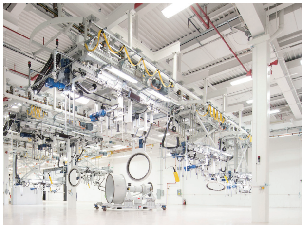
图3 Pratt & Whitney发动机公司建立的发动机装配脉动生产线 Fig.3 Pulse production line for engine, built by Pratt & Whitney engine company
