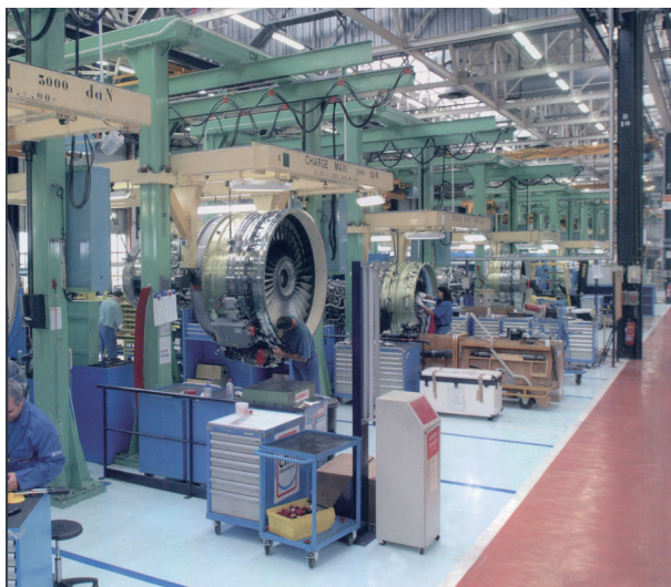
图1 法国斯奈克玛公司采用立式固定框架总装 Fig.1 Final assembly by using vertical mounted frame in Snecma
